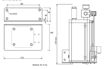
A free space of 300 mm is required above the unit for unobstructed filling. All dimensions in mm.
