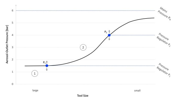
In the case of a tool with large cooling channels (x-axis, left), a low aerosol dynamic pressure occurs at the tool. The aerosol generators work according to the characteristic curve in the operating case 1 with a large differential pressure (between mains pressure  $P_N$  and dynamic pressure) and consequently supply an increased aerosol quantity suitable for the tool.
